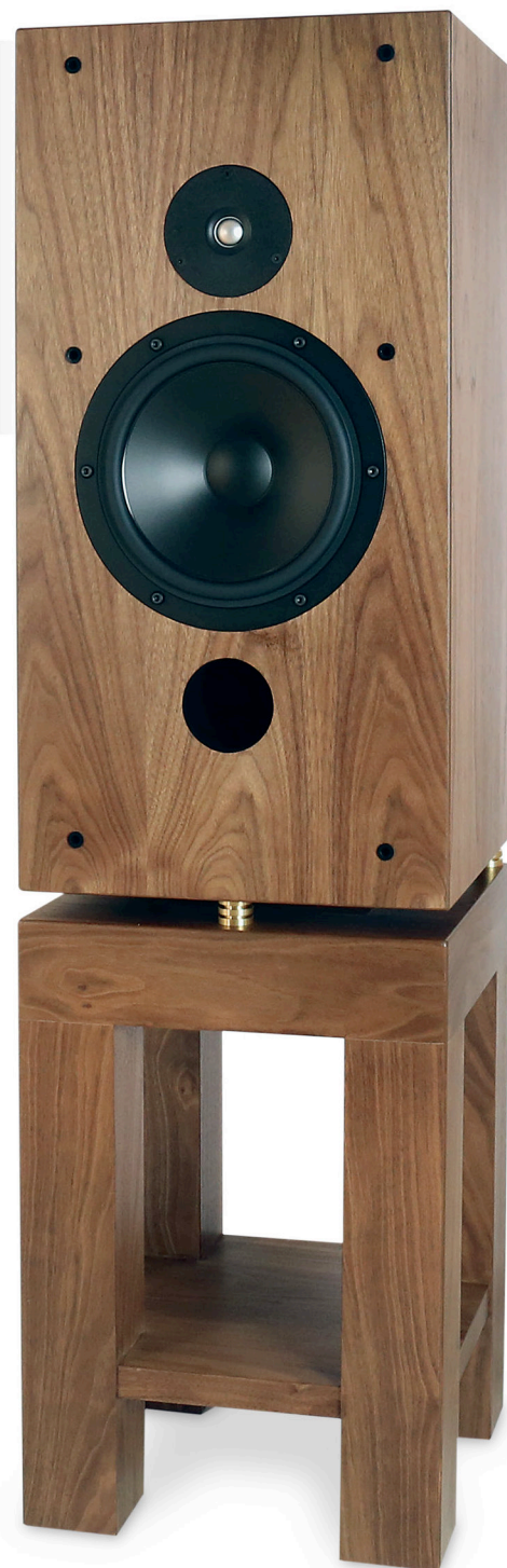
ABOVE: A soft-dome 'platinum coloured' 20mm Hiquphon 3/4 OW4 tweeter is paired with a 230mm C-Quenze driver from AudioTechnology, reflex-loaded through a large, front-facing port
